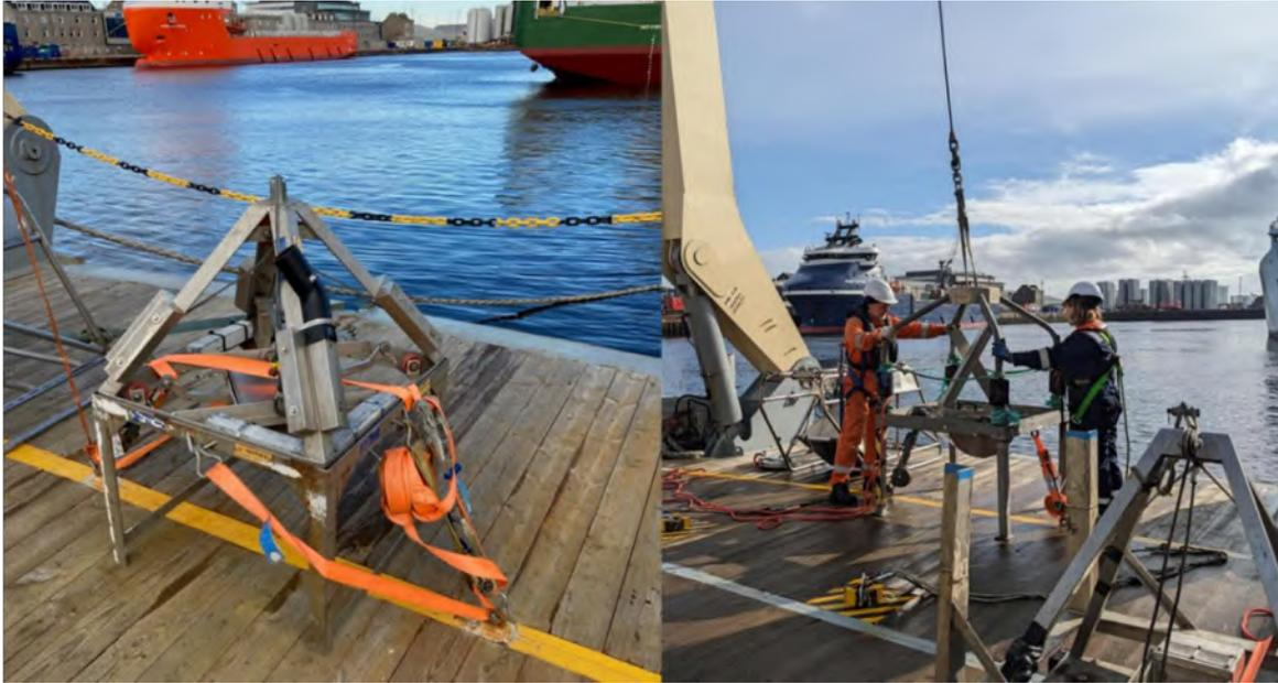
**Plate 4** Left: OEL's 0.1 m<sup>2</sup> Day grab sampler fastened to the aft deck of the *MV Situla*. Right: OEL's 0.2 m<sup>2</sup> DVV grab sampler being deployed as part of wet testing from the aft deck of the *MV Situla*.
