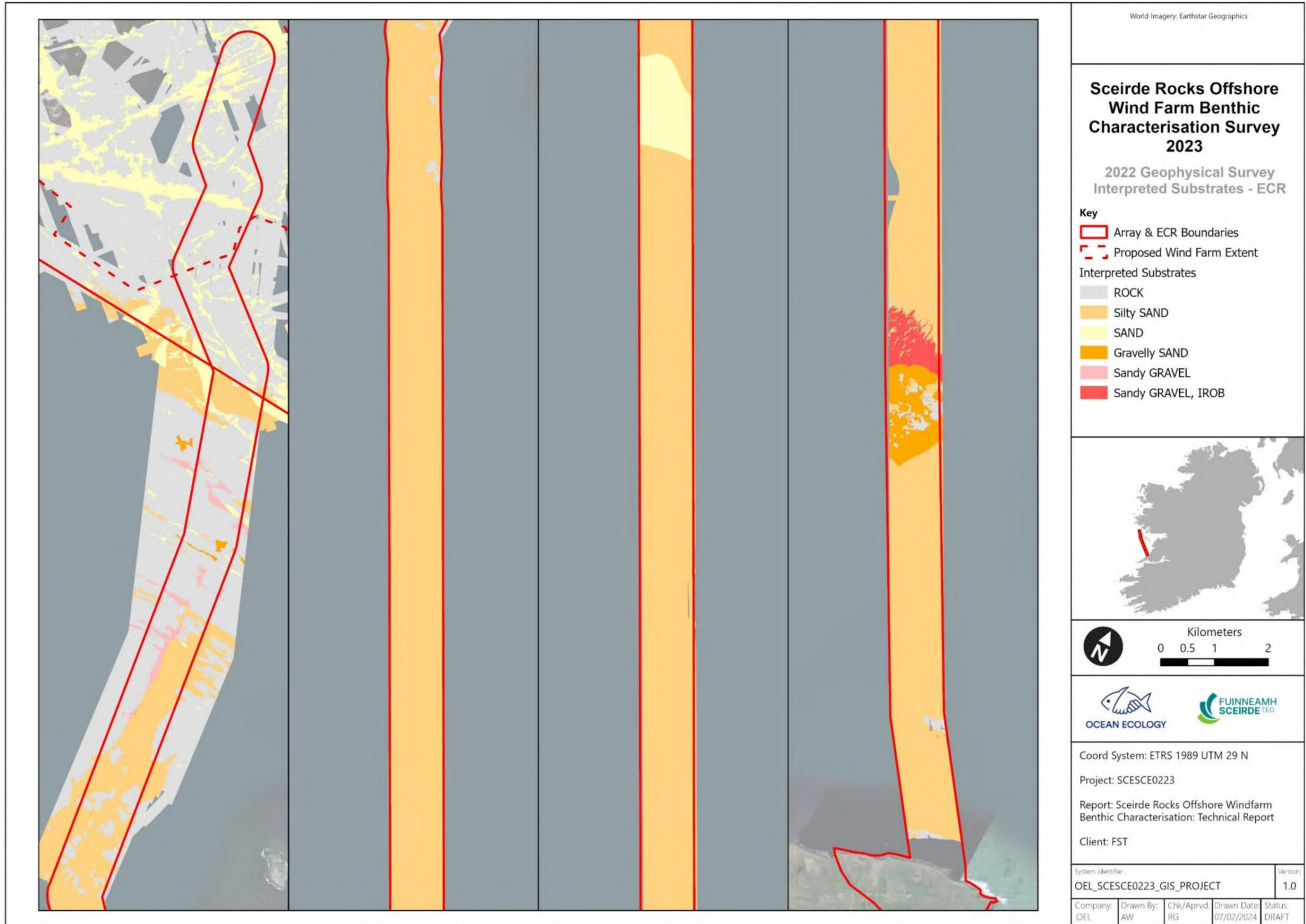
Figure 6 Interpreted substrate from data acquired during the 2022 geophysical campaign (ECR).
