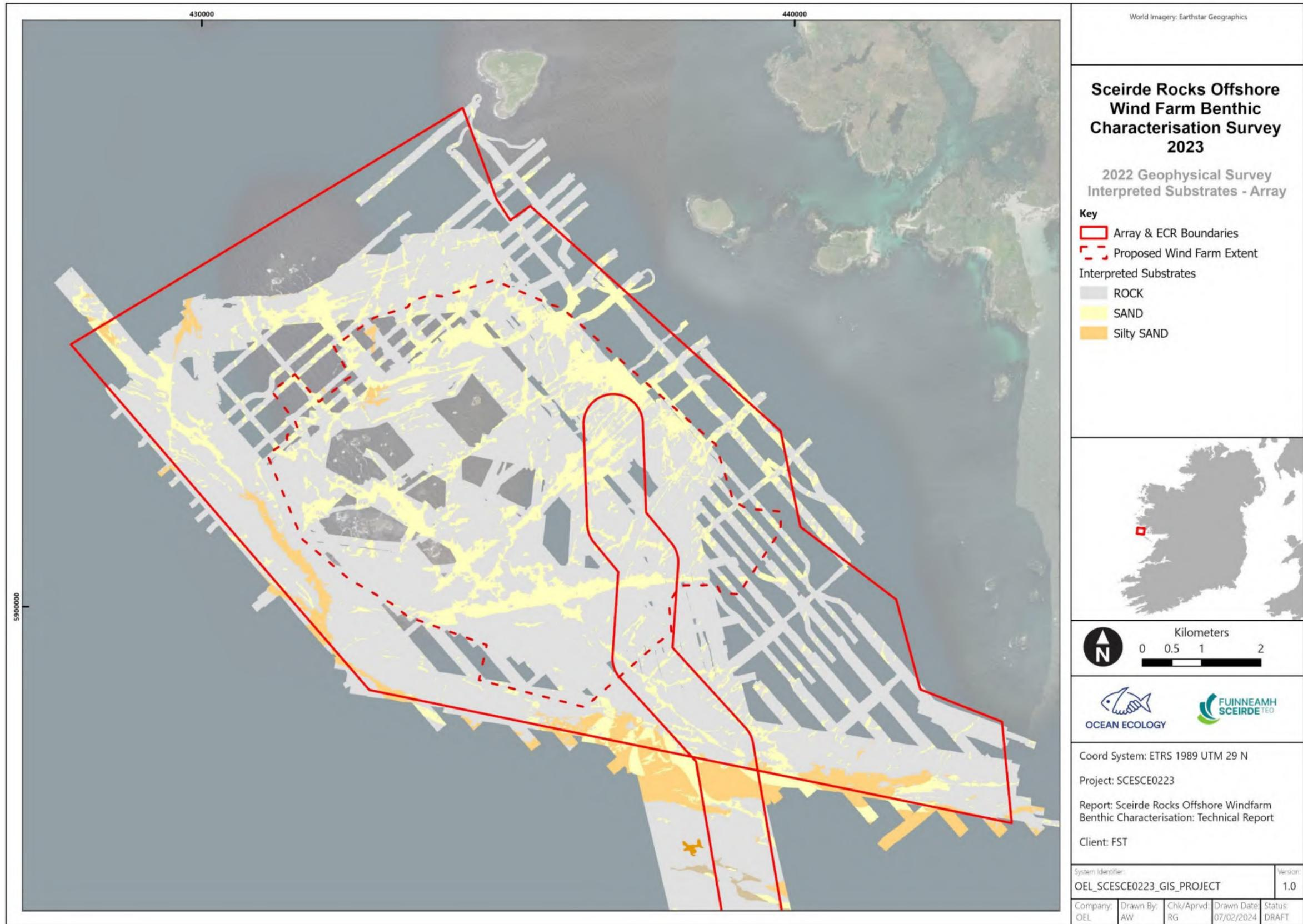
Figure 5 Interpreted substrate from data acquired during the 2022 geophysical campaign (Array).
