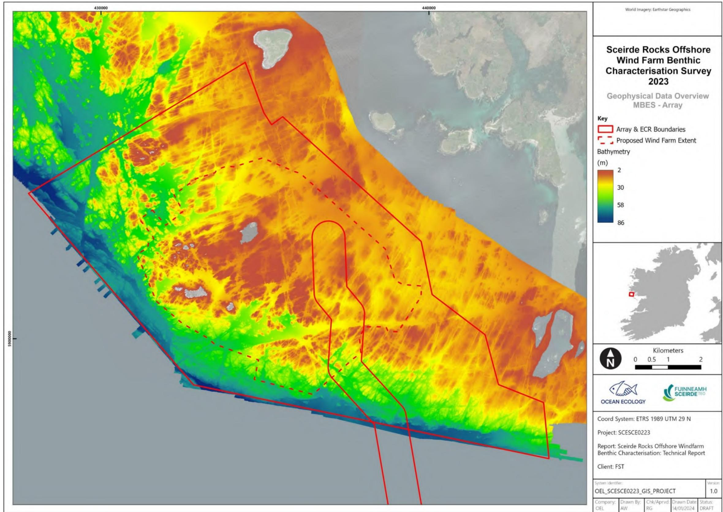
Figure 12 MBES data acquired during the 2022 geophysical campaign (array).
