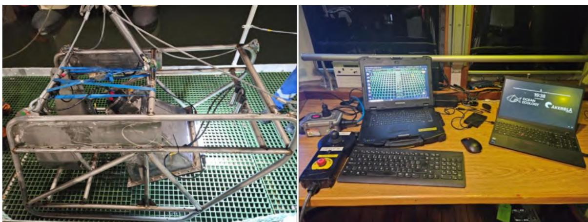
**Plate 3** Left: OEL CLOC camera system. Right: The camera system topside setup.
