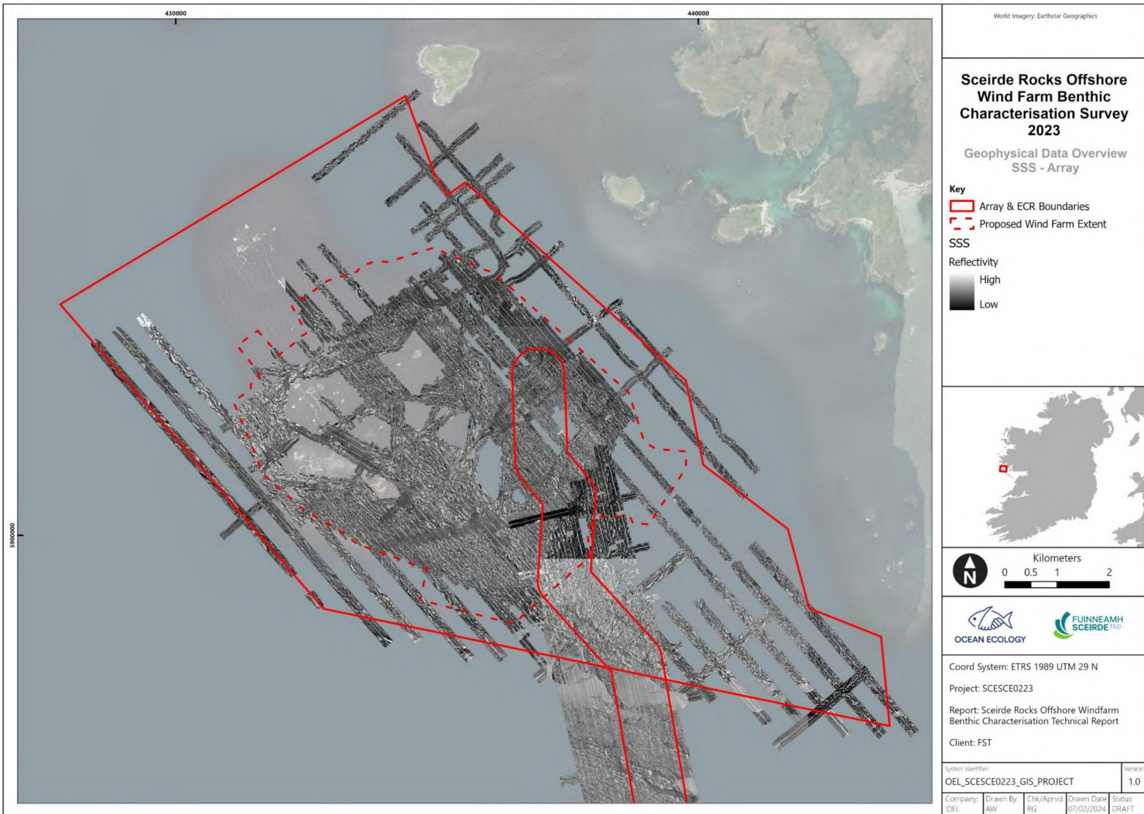
Figure 11 SSS data acquired during the 2022 geophysical campaign (array).
