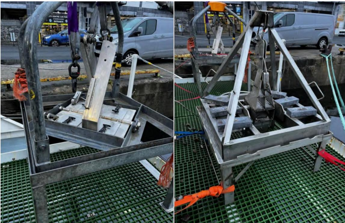
**Plate 5** Left: OEL's 0.2 m<sup>2</sup> Dual Van Veen grab sampler on the deck of the *MV Roman Rebel*. Right: OEL's 0.2 m<sup>2</sup> mini-Hamon grab sampler, mobilised as a redundancy sampler.
